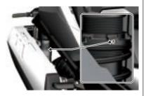
2.Looking down from the top of the shock absorber, rotate the precompression adjusting seat clockwise, and the spring pre-tightening force increases (becomes hard). The spring preload is reduced (softened) by rotating the spring counterclockwise. Tighten the locking screw after adjustment, and continue to tighten 1/2 to 3/4 turn when resistance is felt.
