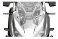
1. Remove the two expansion pins on the head cover and remove the head cover.
