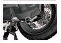
1.As shown in the figure above, check whether the waste oil pipe of the air filter accumulates dirt or water. If dirt or water is found, remove the clamp in the figure below with a caliper, pull out the black plug, and reinstall the plug after draining the waste oil and sewage.
