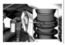
3.The adjustment knob for restoring the damping of the rear shock absorber can be rotated by hand. The adjustment range is 7 gears. The standard position is to rotate the knob to the end in the "+"direction and then rotate it to the fourth gear in the"-" direction.Rotate in the "+"direction to increase the restoring damping (stiffen), and rotate in the"-" direction to decrease the restoring damping (soften).
