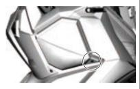
1. Disassemble a swelling nail on the outer lid of the right front box and remove the outer lid of the right front box.
