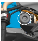
Main water tank cover
